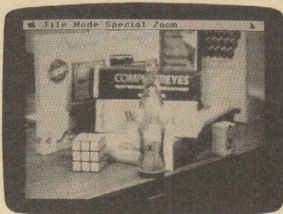
Here, several Apple software packages have been digitized using AST-VisionPlus's black-and-white mode.
