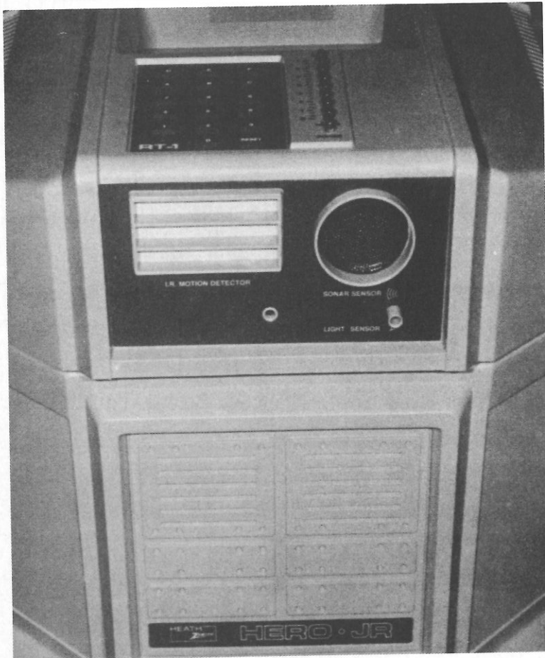
Fig. 8-3. A Heath HEROjr personal robot. A 17-key keypad, located on the top of HEROjr's head, is used for direct robot programming. An RS-232C port on HERO's back, however, provides Apple IIGs access to all levels of personality programming that are possible with this robot.
