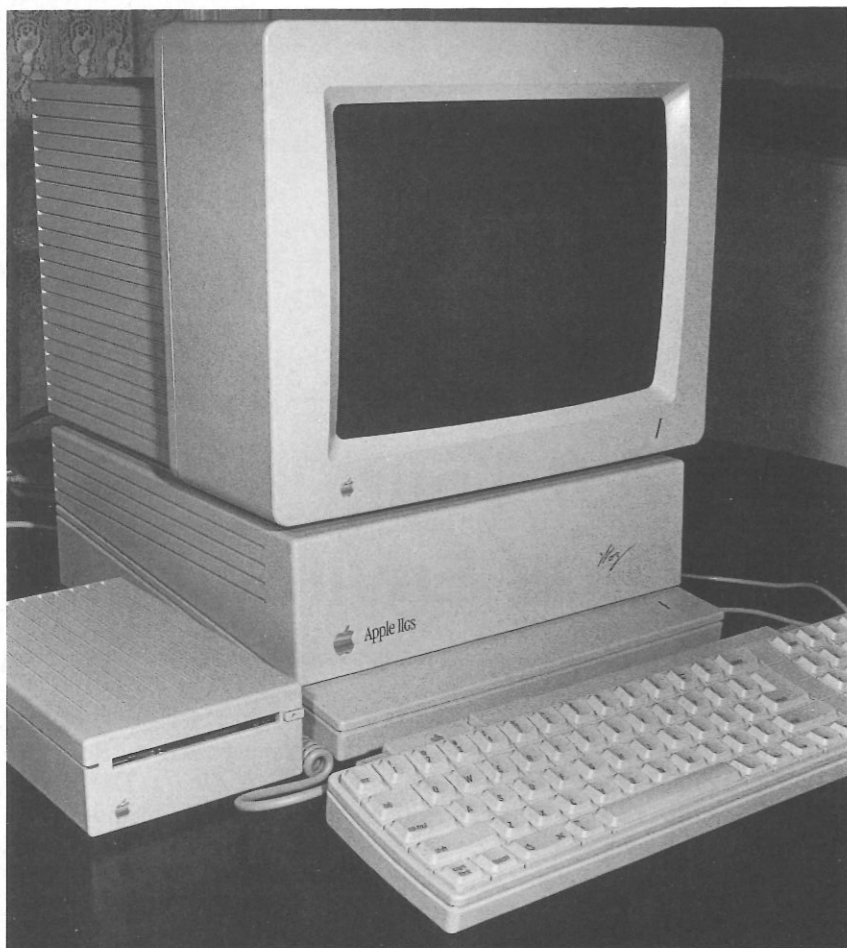
Fig. D-1. The main Apple IIgs housing. The mouse is not visible in this picture.
