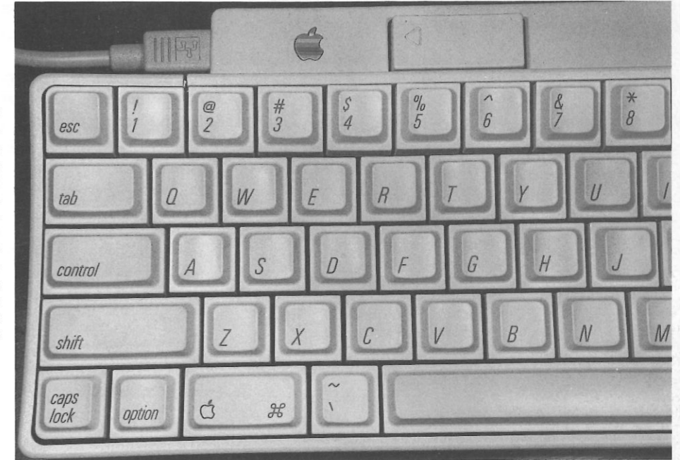
Fig. D-6. One of many new hardware features on the IIgs is the Apple DeskTop Bus port which is located in the detached keyboard. Two other interesting features in this figure are the combined Open-Apple and Command keys (lower left corner under the Z key) and the Reset button (above the 5 and 6 keys).
