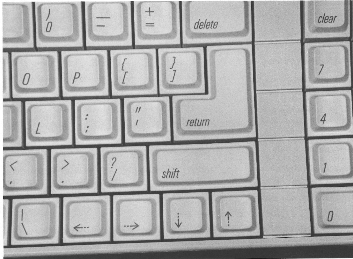
Fig. D-2. Just like the keyboard on the Apple IIe and IIc, four arrow or cursor keys are located under the right shift key on the IIGs.
