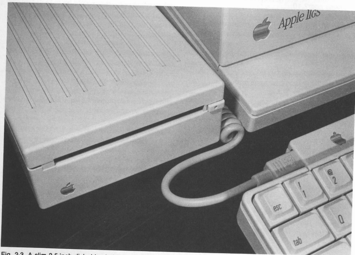
Fig. 2-3. A slim 3.5-inch disk drive holds up to 800K bytes worth of information.
