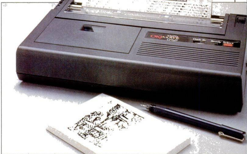
Okidata's Okimate 10 uses thermal-transfer technology to provide four-color printing at a cost to the user of about 66 cents a page, approximately the same cost as duplicating a color slide.
